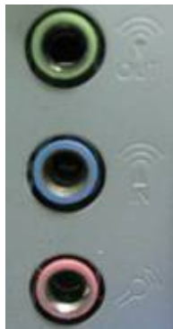
Fig 1-B-1 A typical sound card connector panel
